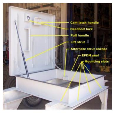
Custom sizes are available - we've built manually operated hatches up to 36" x 144" that are fully insulated with a zinc rich "cold galvanizing" primer finish, a topcoat of paint, and an automatic hold open device. To find out more, contact our sales department at 541-459-1806 or sales@AmericanSafeRoom.com.
